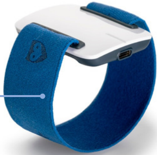
Wearable sensor that detects seizures using Photoplethysmography (PPG) and Accelerometry (ACC) sensors
